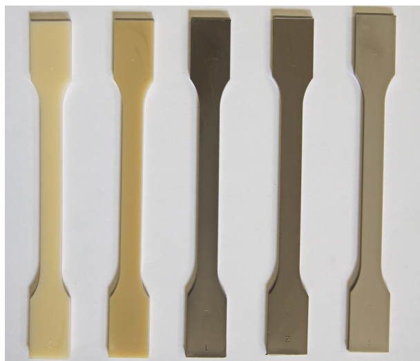
Fig. 1. Multipurpose test specimens according to ISO 3167.
