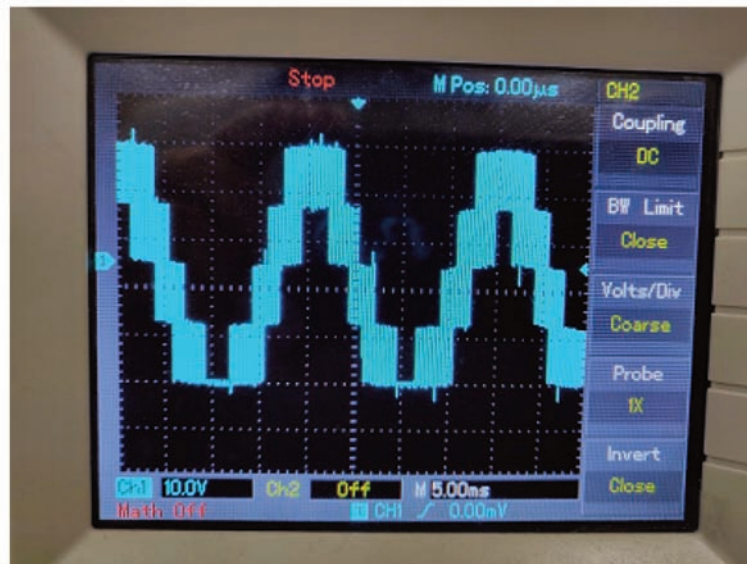
Fig. 18. Generated voltage in Phase A without a filter.
