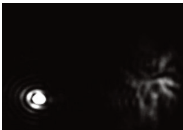
Fig. 4. Captured image of the formed SrS particles (surrounded by a series of diffraction rings) in MilliQ water in the NTA video frame.
