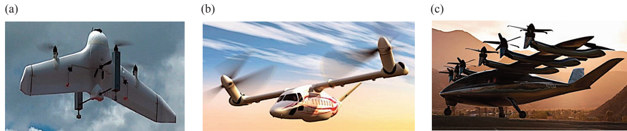
Fig. 1. Design examples of (a) tail-sitter [8], (b) tiltrotor [9], and (c) tiltwing [10] vertical take-off and landing (VTOL) aerial vehicles.
