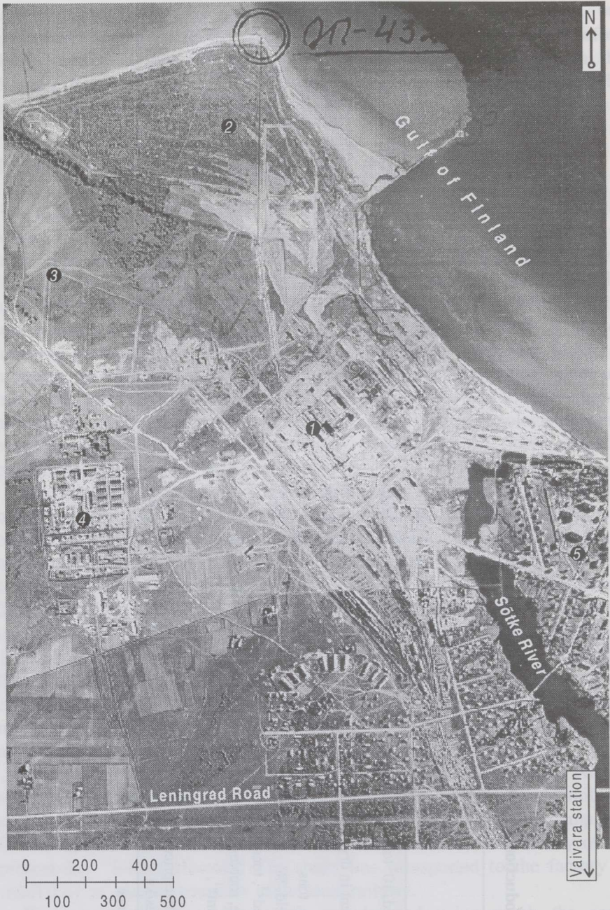
Aerial photo of Sillamäe in 1951. The uranium factory "Plant No. 1 of Combine No. 7" is located in the centre of the picture (1). Just North of it is the waste disposal area at the sea (2), and the underground mine extends NW from the factory to the sea (3). The prison camp is the rectangle West of the factory (4). Living quarters and barracks for the workers are located South and SE (town centre) from the factory (5)
