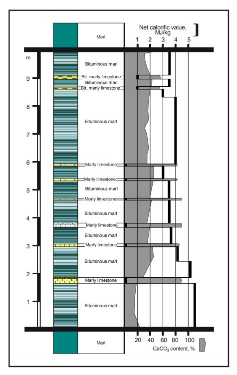
*Fig. 1.* Geologic section of the Dotternhausen oil shale deposit showing the variation in CaCO<sub>3</sub> content and net calorific value
