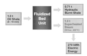
*Fig. 5.* One process (fluidized-bed unit) – two products (hydraulic burnt shale + electric energy)
