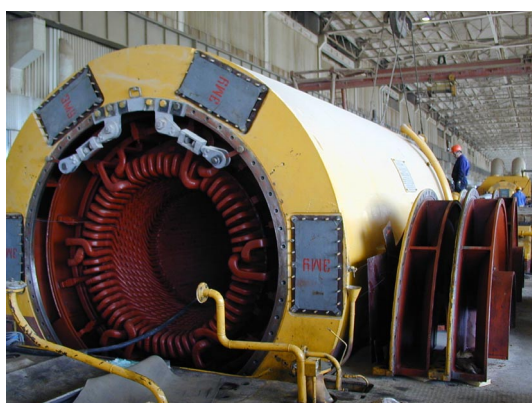
Fig. 3. Search for hot spots by hand and pyrometer
