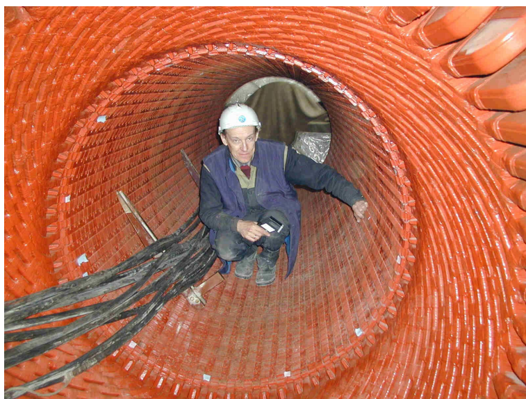
Fig. 3. Search for hot spots by hand and pyrometer
