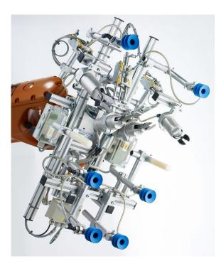
Fig. 4. End of arm tooling [8].
