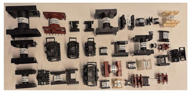
Fig. 7. Dividing parts according to the gripping surface area.
