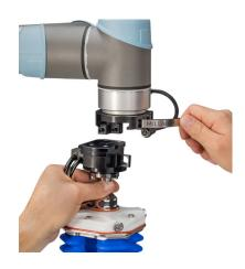
Fig. 2. Manual tool changer [6].
