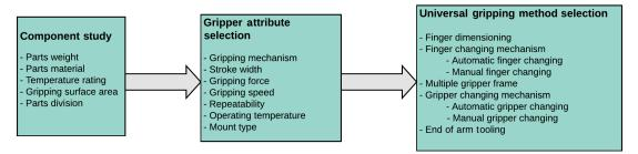
Fig. 6. Process flow for achieving universal gripping.
