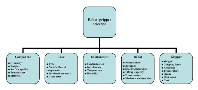
Fig. 5. Governing factors for gripper selection (adapted from [2]).
