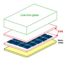
Fig. 1. Layers of solar module [8].
