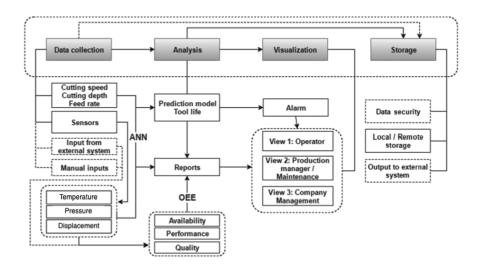
Fig. 2. Concept of the production monitoring system [18].
