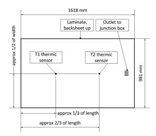
Fig. 3. Schematic representation of experimental setup.
