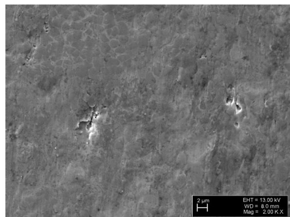
Fig. 6. Topography of the wear surface after ARWW of \text{Cr}_3\text{C}_2\text{-Ni} .
