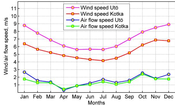
Fig. 2. Monthly mean wind speed and average air flow speed at Utö and Kotka during 1981–2010.
