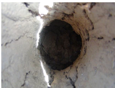
Fig. 3. Field test on the farmland (90 kJ once).
