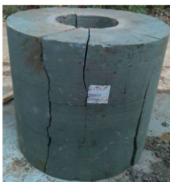
Fig. 2. Laboratory test on the sandstone sample (30 kJ for five times).
