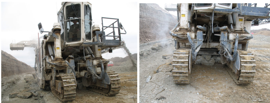
Fig. 4. Effect of cutted rock oversizing in case h/V ratio >6\% .
